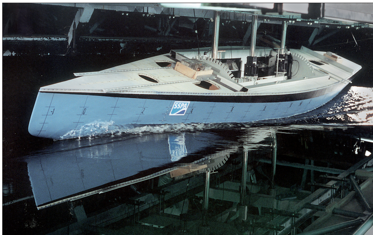
Fig 17.5 IACC hull under test at SSPA in Gothenburg (Photo: SSPA)
