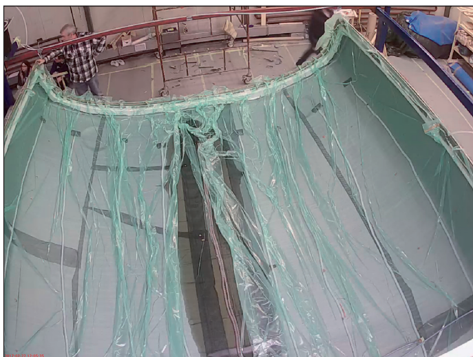
Fig 15.49(a-c) (TOP TO BOTTOM) Infusion process – growing dark area shows the progress that resin makes through the material
