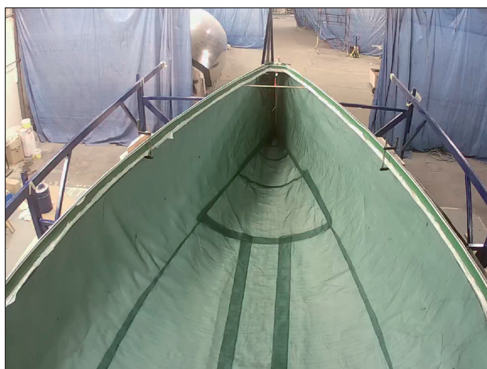
Fig 15.46 (ABOVE) Dry reinforcement and sandwich materials laid in the mould
