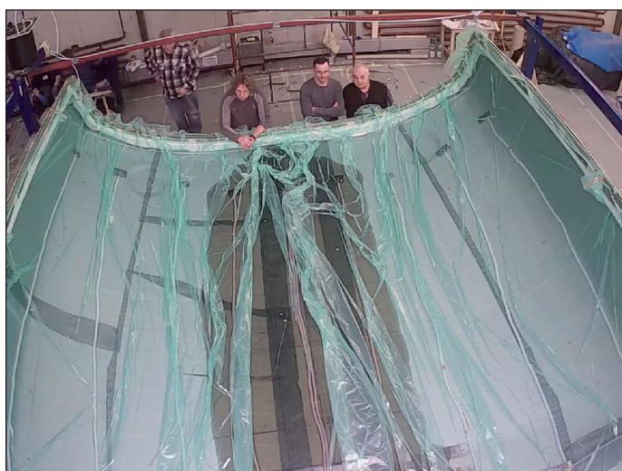
Fig 15.49(a-c) (TOP TO BOTTOM) Infusion process – growing dark area shows the progress that resin makes through the material
